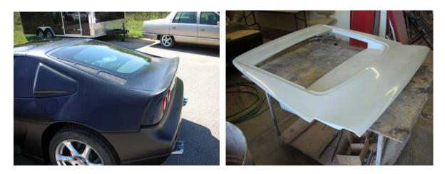
About a year ago, at the request of a customer, V8 Archie designed a hatchback conversion for the '86-'88 Fiero GT. This hatchback conversion, now available as a "kit", requires no modifications to the original Fiero GT rear clip and is basically a "bolt on" unit. Made of fiberglass, the kit consists of an outer & interior skin, bonded together with steel reinforcement ribs to provide a solid OEM type fit, finish and quality.
