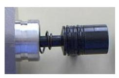
Same top quality construction as the Getrag V-6 5-speed slave shown above, but fits the 5speed Isuzu ('85-'88 4 cylinder) and the Muncie 4-speed used in the '85-'86 V6 Fiero. (Note: Rodney does not currently offer a slave cylinder for the '84 4 cylinder, 4-speed Fiero, but will soon). This aluminum slave also sells for \$79.95 and like the V6 5-speed Getrag slave it also features the double seal piston!
