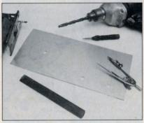
Cut out the panel to the desired shape. With a pencil, mark the location of instruments, switches, and mounting holes. Use a punch to mark the centers and then drill the holes to size. Use a compass with a soft lead to mark larger holes. If a saber saw is needed to cut instrument holes, cut from the backside or lightly glue cardboard to the metal to prevent scratching the surface.
