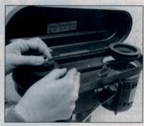
Set the drill press for its slowest speed (900 to 1,400 rpm). Most drill presses have a multiple-size pulley arrangement that allows the belt to be switched from one pair of pulleys to another to alter the speed.
