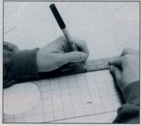
To draw a grid on the dash, use a soft, fine-tip marking pen (so as not to scratch the surface). The squares should be slightly smaller than the turning-tool's diameter. For ½-inch swirls, make the squares ¾ inch. For 1-inch swirls, use ¾-inch squares. Experiment on scrap first, as you may prefer more or less overlap than this. For more overlap, make the grid smaller.
