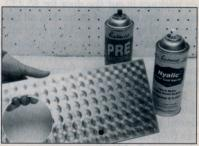
Clean thoroughly with a paint-prep solvent like Eastwood PRE aerosol. Then coat with a clear coating like Eastwood Nyalic Clear Coat Barrier to keep your masterpiece from losing its luster. Engine-turning adds a hand-finished touch that complements any kit project. **KC**
