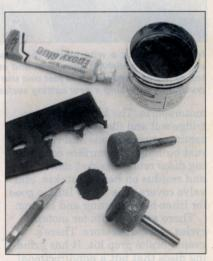
For a handmade tool, glue a thick leather circle to a same-size grinding stone (use strong epoxy). Trim the leather to tool size. You'll need valve-grinding paste too. We recommend that you make several tools in case one comes unglued while you're working. Old belt leather or shoe leather works great.
