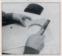
The part mustn't have scratches or dents. Sand it with 360-grit wet/dry sandpaper until it's smooth. File the edges and bevel the screw holes to avoid damaging the turning tool.
