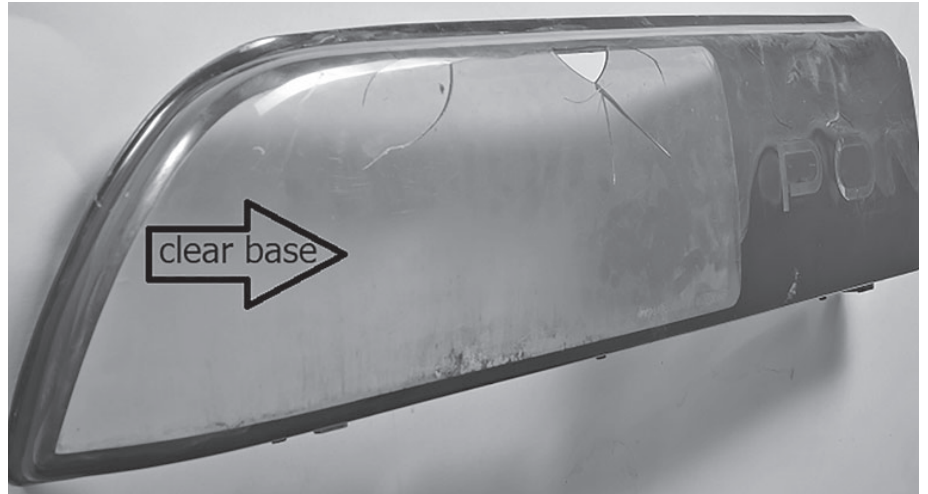
(Image 3) Typical OEM lens cover after 30 years
