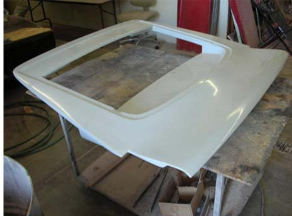
About a year ago, at the request of a customer, V8 Archie designed a hatchback conversion for the '86-'88 Fiero GT. This hatchback conversion, now available as a "kit", requires no modifications to the original Fiero GT rear clip and is basically a "bolt on" unit. Made of fiberglass, the kit consists of an outer & interior skin, bonded together with steel reinforcement ribs to provide a solid OEM type fit, finish and quality.
