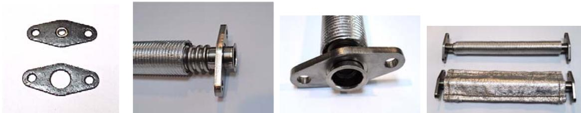
One of the most frustrating Fiero V6 failures is the EGR tube that attaches under the intake plenum and connects to the base of the EGR valve. Over time, as the engine vibrates, the weld at the flange joints fail and a vacuum leak becomes apparent as a faster idle. Rodney Dickman now manufactures OE replica EGR tubes for both the '85-'87 V6 and also the '88 V6 (Image 1).
