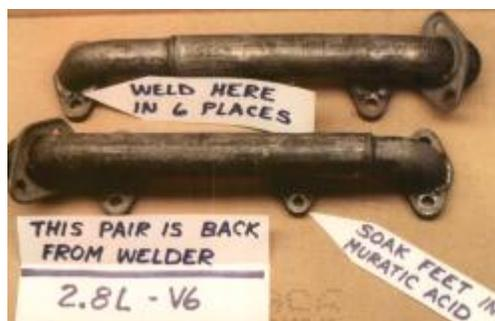
Common symptoms for a cracked manifold can be a loud engine exhaust sound, similar to a bad muffler. Another symptom can be a ticking sound from the engine. This sound can give you the impression that the engine itself has an internal problem. In reality, the engine is fine, but the exhaust leak through the crack causes the engine to "tick".
