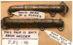
Common symptoms for a cracked manifold can be a loud engine exhaust sound, similar to a bad muffler. Another symptom can be a ticking sound from the engine. This sound can give you the impression that the engine itself has an internal problem. In reality, the engine is fine, but the exhaust leak through the crack causes the engine to "tick".
