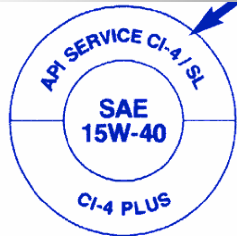
A 'cross-over' diesel oil, formulated for both diesel engines (CI-4) and gasoline engines (SL).
