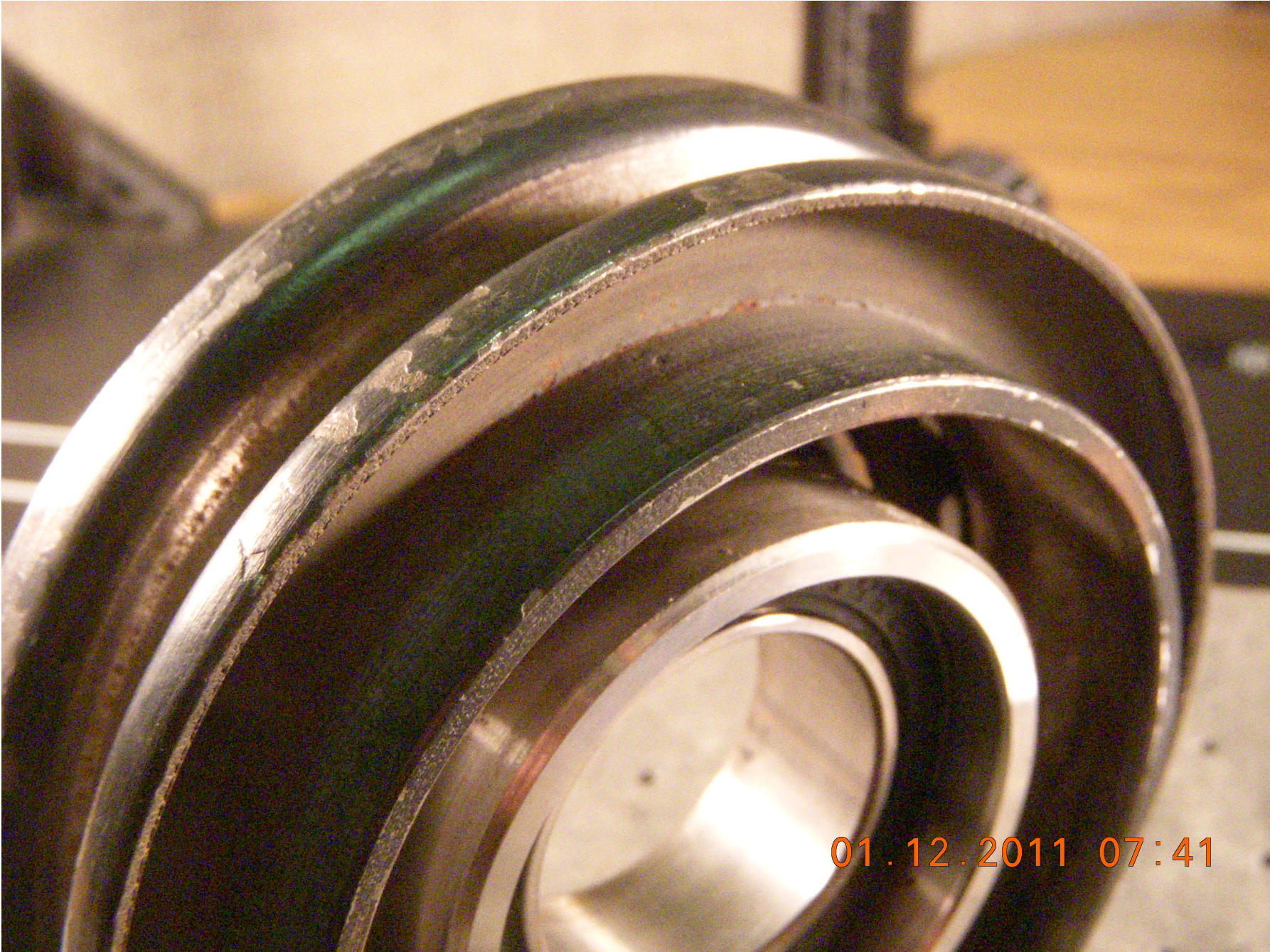
ROTOR OUTER POLE/SPUN PULLEY JOINT – PROBABLY ENERTIA WELDED
